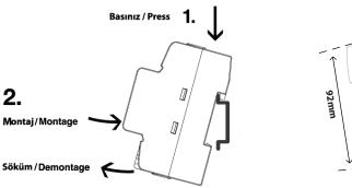
After hanging the upper part of the device onto the rail, push the lower part towards the rail until you hear a clicking sound. To remove the device from the rail, first push it downwards and pull the lower part towards yourself, releasing it from the rail, then gently push it upwards to remove it from the hanging position.
